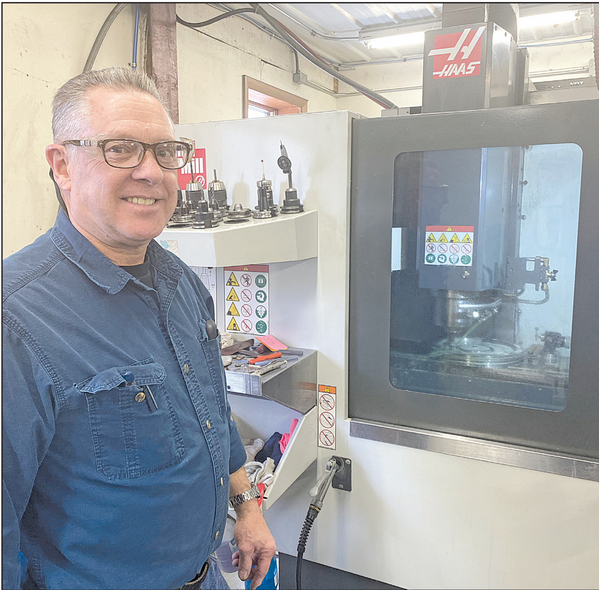
Chenango Valley Technologies employee Jim Peckham is monitoring a HAAS CNC milling machine as it cuts new mold components. (Photo by Kelli Miller)
